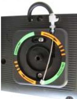
...and fasten the base of the release knob to the side panel using 2 self-threading screws.
