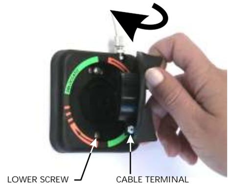
Now, insert the release knob on the base of the mechanism, being careful to keep the cable terminal in the seat of the cable block and the knob in the correct position. When inserting the knob, the cable terminal must be in the position just beyond the lower fastening screw, in a clockwise direction.
