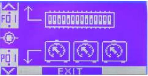
To set the functions relative to the dip switches, briefly press the F01 **F2** button (see paragraph 6a).
