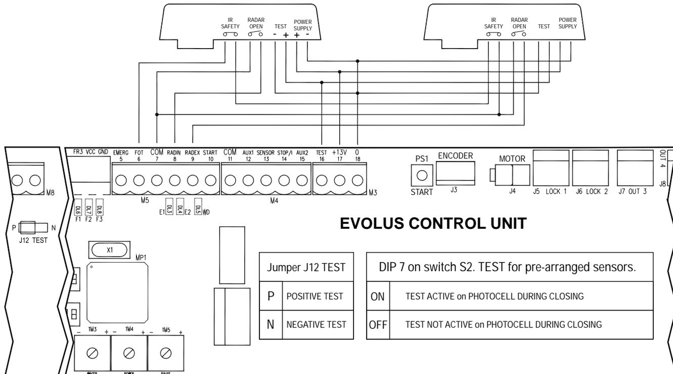
The diagram illustrates the connection on the operator of two sensors with twin outputs and monitoring test to detect movement (radar) and presence (safety photocell).
