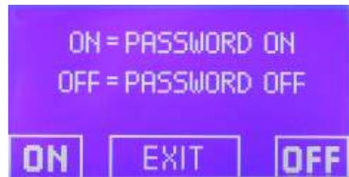
If the ON button is pressed, a screen will appear on the display where the new password is requested. Now enter the desired password, selecting a combination of 5 characters from the letters A-B-C-D. To select the letters, press the button in correspondence of the letter itself.
