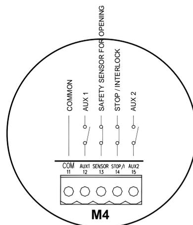
**13** = input of the Safety side sensor for opening; N.C. contact.
