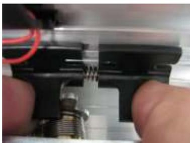
Position the second and third plastic release components as shown in the figure, making sure that the stroke of the third component is sufficient to activate the lever on the electric lock. Fasten the second component into position with self-threading screws.
