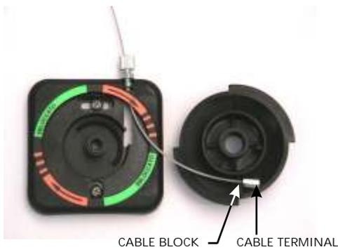
Pass the release cable in the slit in the base and then inside the adjustment register as shown in the figure. Then position the cable terminal on the release knob cable block (see figure).
