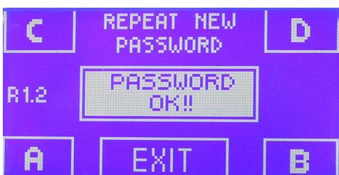
The system will now automatically return to the main programming menu. Press the ENTER
