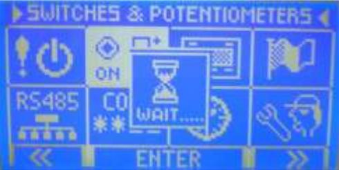
Press the **F1** button until the
