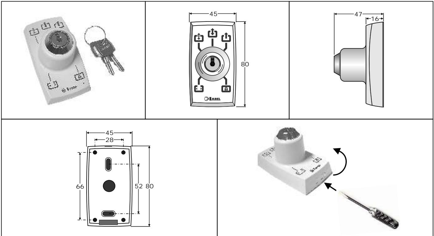
The **EV-MSEL** key mechanical selector permits to setup the work program of the automatic EVOLUS door. To enable its operation set dip 6 of S1 to ON (see paragraph 14).
