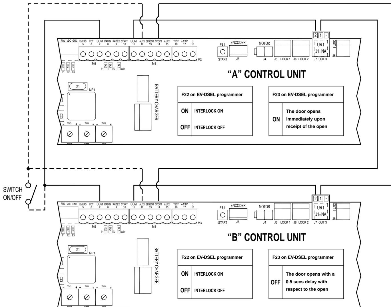
**The dotted line of the ON/OFF switch connected to the AUX/1 input is used to disable the interlock operation (connection not essential for the system operation).
