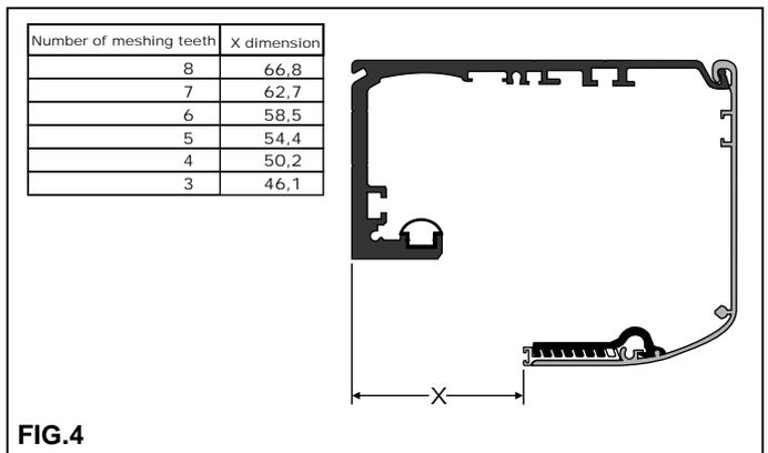
Choose the optimum adjustment depth for the compensating profile referring to Fig. 4 then fasten each plastic clip by first inserting the clip teeth into the compensating profile grooves and then pushing the upper section of the clip forward until it connects to the casing.
