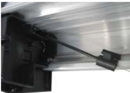
Insert the plastic release components as shown in the figure, considering that 4 plastic components are necessary to install the manual release on the left side.
