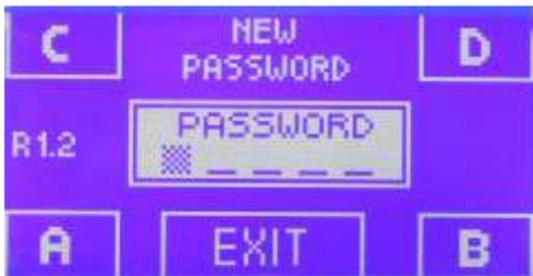
After entering the password the first time, the combination must be repeated a second time. Enter the previous password again.
