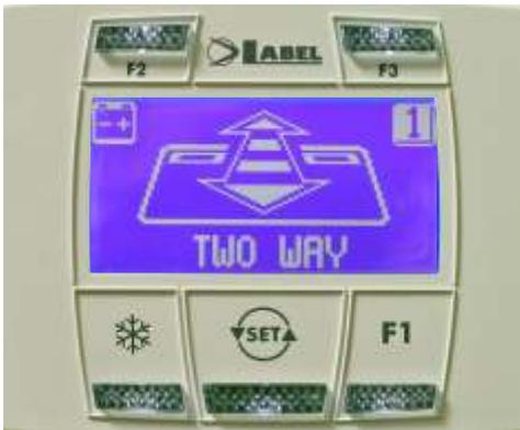
If the symbol
