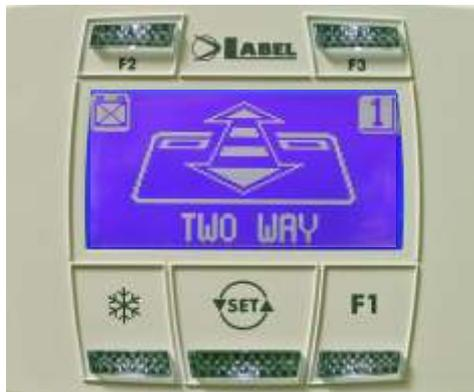
If the symbol
