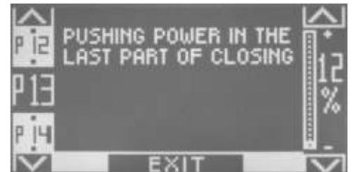
**P14 = Thrust power at the end of the closing cycle**
