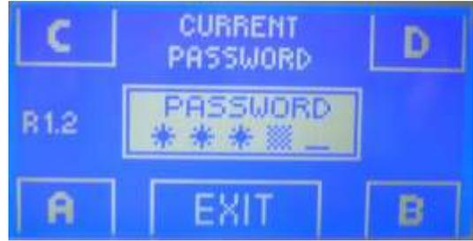
Press the button in correspondence of the letter "A" a fourth time, and an asterisk will appear on the display in the field for the fourth letter.
