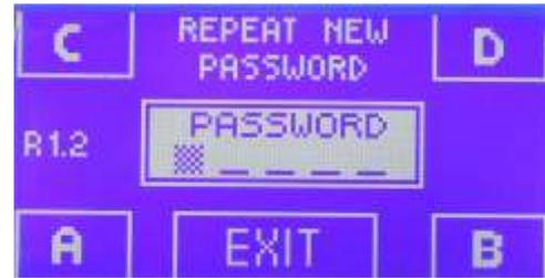
If the entered password is correct, the message "PASSWORD OK!!" will appear on the display.
