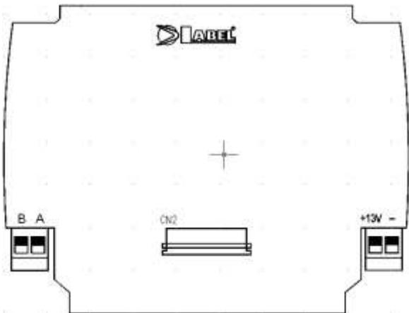
Connect the digital programmer EV-DSEL to the electronic control unit for the EVOLUS door using a 4 pole cable with a diameter of 0.5 mm.
