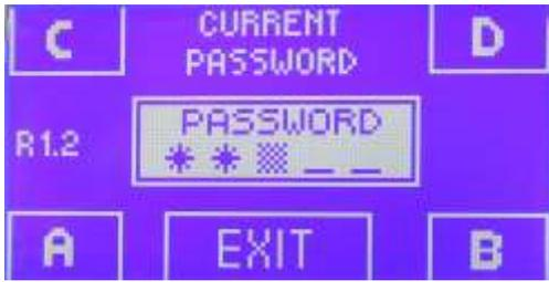
Press the button in correspondence of the letter "A" a third time, and an asterisk will appear on the display in the field for the third letter.
