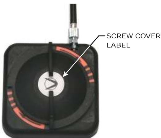
Once the knob is inserted, fasten the closing screw, insert the sheath and turn the knob to the UNRELEASED position. In this position, only the orange part of the label must be seen with the drawn black arrows.
