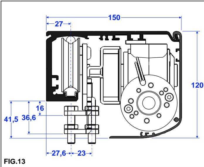
The transom must be fastened to a flat surface solid enough to bear the weight of the leaves to be used. If the wall or the support do not meet these characteristics you will have to provide for a suitable tubular element, as the transom is not self-bearing.
