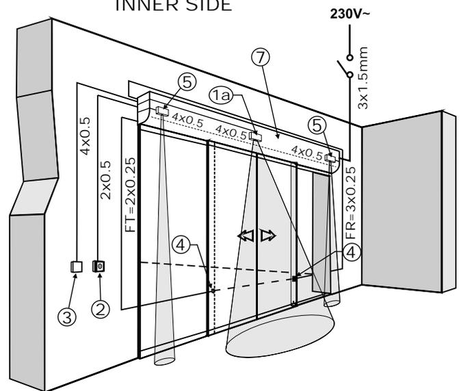
Notes: The grey part identifies the radar and sensor detection area. For each device the picture indicates the number of cables and the relevant section in millimetres.
