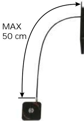
Identify the fastening point on the wall, considering that the standard cable sheath is 50 cm long.
