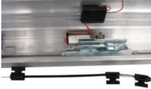
A 250mm sheath must be placed between the second and third plastic release components and the compression spring between the third and the fourth.
